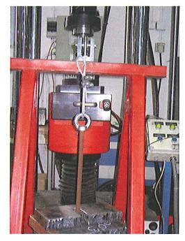
Vertical load test: The load for this test must be three times the maximum service load obtained from the most unfavourable combination of the following values:
